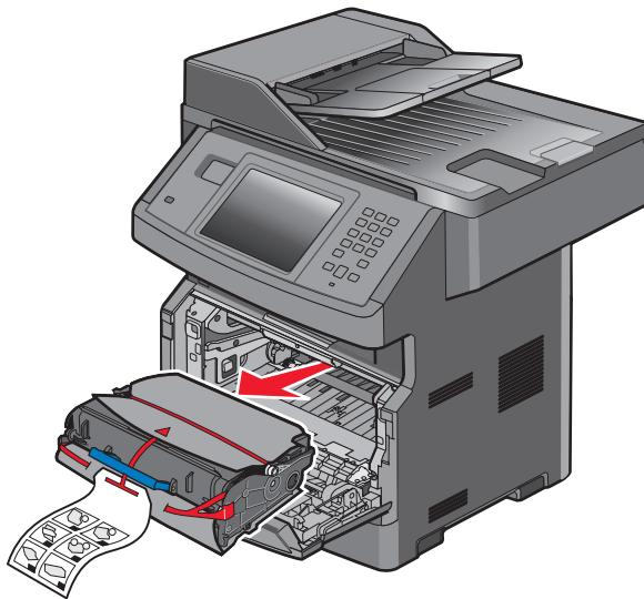
Remove the photoconductor kit and toner cartridge.
