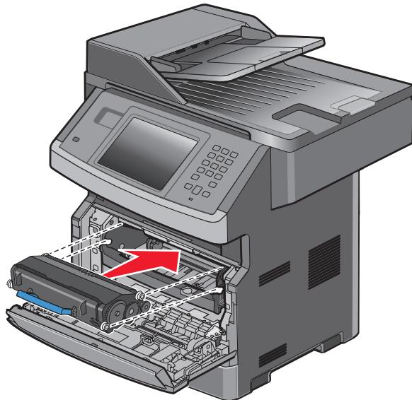
Insert the photoconductor kit and toner cartridge.
