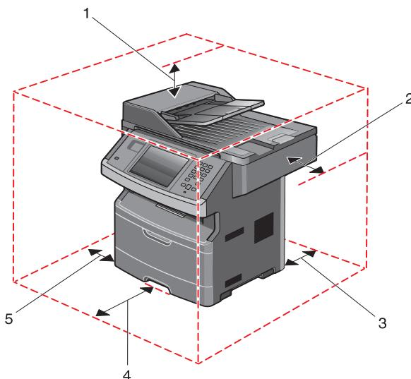
When the printer is set up, allow clearance around it as shown.
