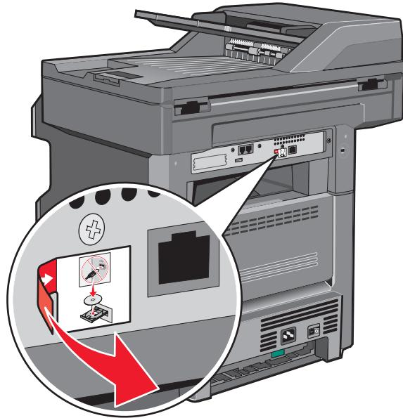
Remove the yellow label covering the USB port. Connect the USB cable to the printer and the computer.
